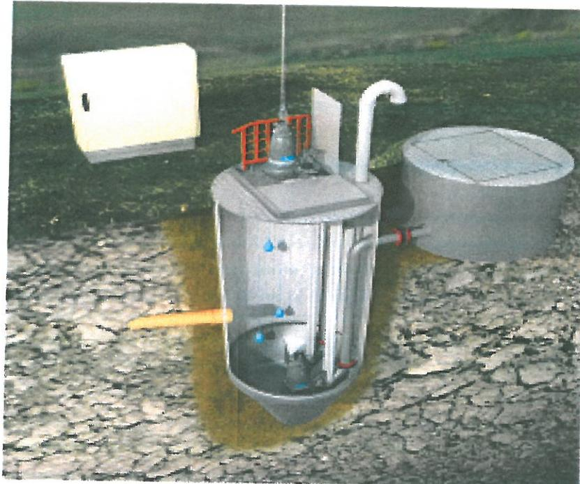
Wastewater flows into the tank from homes and industries. It is then pumped to a higher elevation through pipes and discharged into a gravity flow line that will carry the wastewater to the sewage plant.
