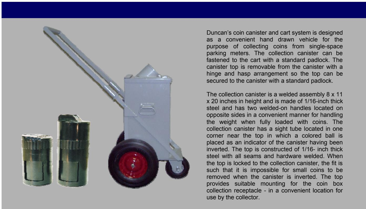
The cart chassis is constructed of 10-gauge steel with bracing and axle retainer all welded in fixed positions with no bolted parts. The pull handle is hinged to allow folding for transport and can be locked in the extended position by a sliding steel tube. The cart has two 12-inch diameter wheels with 3-inch wide semi-pneumatic tires mounted on a 3/4- inch diameter steel axle, and a single 6-inch diameter wheel with a 2-inch wide semi-pneumatic tire mounted on a 3/4-inch diameter steel axle.
